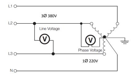
In a star or wye-connected system, the line voltage is higher than the phase voltage by a factor of the square root of 3 (1.732).
