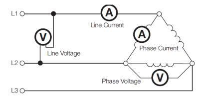
In this configuration the line voltage and phase voltages are the same.
